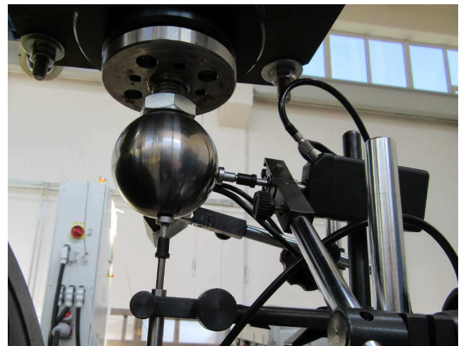
Fig. 5. Measuring sphere and placement of sensors.
