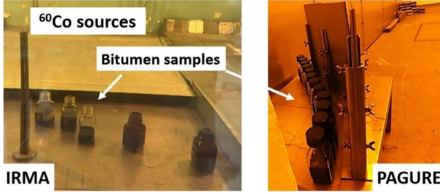
Fig. 1. Bitumen samples irradiated in IRMA and PAGURE facilities.
