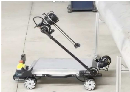
Fig. 14. Prototype 1 in the demonstration to inspect the exterior of a pipe.
