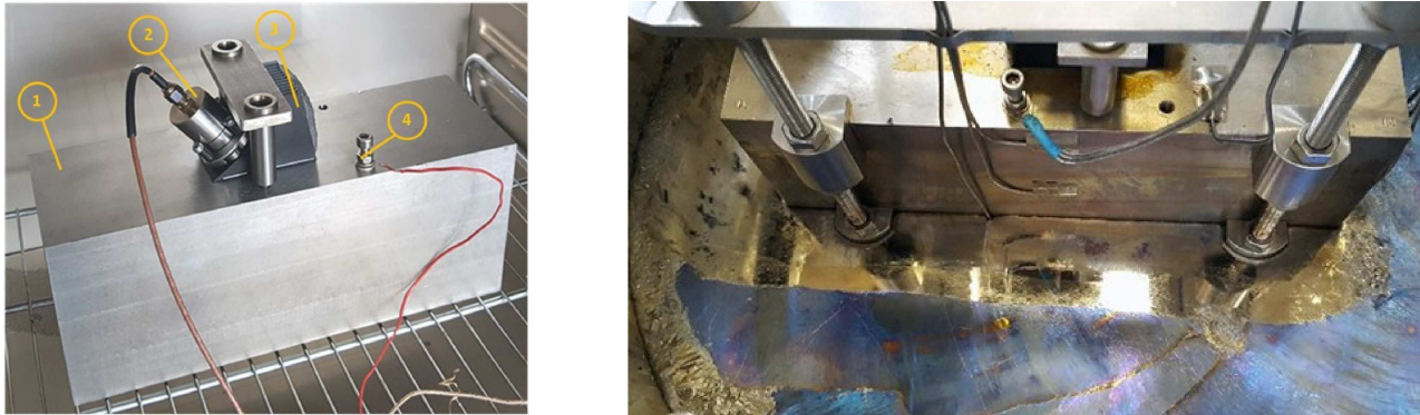
Fig. 11. Ultrasonic sensor installed on the calibration block for tests in air (left), and experimental setup mounted in the LBE vessel (right) (courtesy of KTU). 1 – calibration block; 2 – ultrasonic transducer; 3 – wedge; 4 – temperature sensor.
