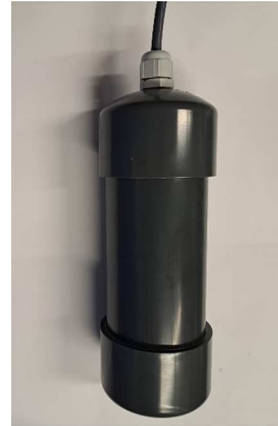
Fig. 2. Example of casing containing the \gamma -detector and ancillary sensor. The length is approximately 10 cm and stands water pressure up to 3 m.
