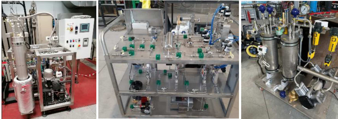
Fig. 12. From left to right, first prototype for gas trapping, design before, and after manufacturing by Air Liquide Italia.
