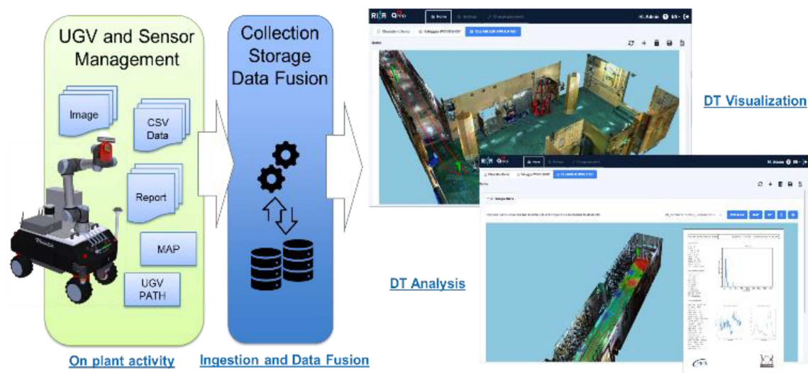
Fig. 15. Diagram of data collection, fusion visualization and analysis for the Digital Twin.
