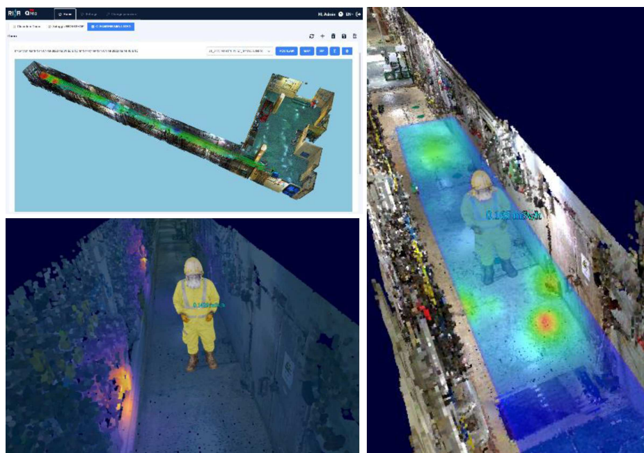
Fig. 17. Orano's poStLAM software and its integration within the QPro platform showing dose rate maps and 252 retroprojections in the tunnel where the demonstration during the final workshop took place.
