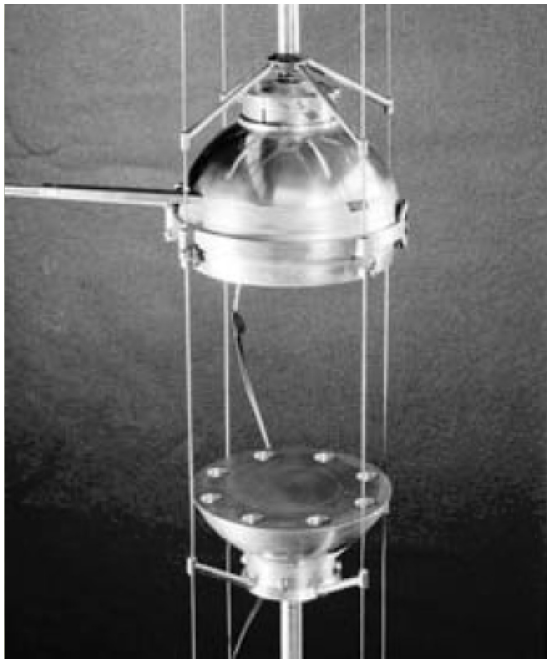
Fig. 2. The Jezebel ^{239}\text{Pu} critical assembly shown above is widely used by nuclear data evaluators to constrain their evaluations of neutron-induced reactions on ^{239}\text{Pu} , creating hidden correlations between different quantities such as \bar{\nu} , PFNS and \sigma_f as discussed by Bauge and Rochman [1] and Rochman et al. [2].
