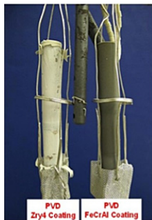
Fig. 8. Mo tubes with both-ends welded to endcaps and coated with either FeCrAl or Zircaloy-4 after testing in 1000^\circ\text{C} steam for 7 days.
